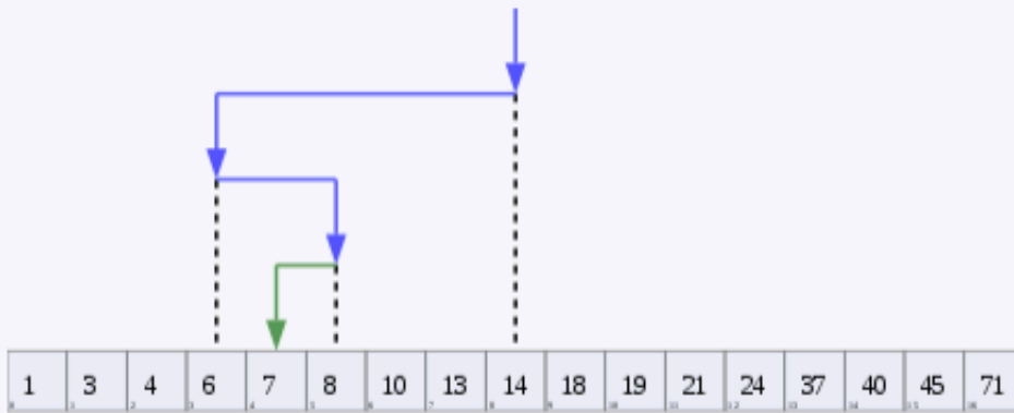
Visualization of the binary search algorithm where 7 is the target value
